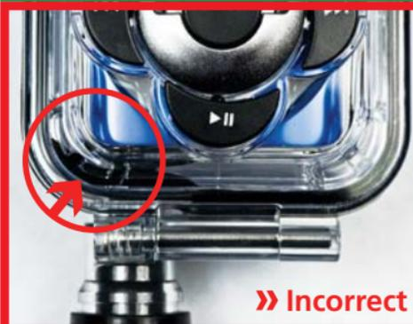
**This seal is misaligned and has been pinched between the base and the lid, creating an opening that will cause the case to flood.**
